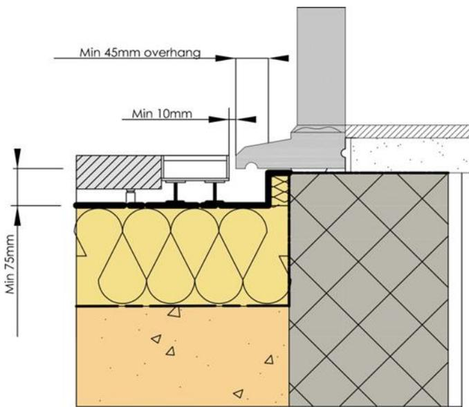
Drainage outlets must be easily accessible and maintainable even if decking / balcony floor finishes are applied. Balcony steelwork must be adequately protected against the potential for corrosion.
