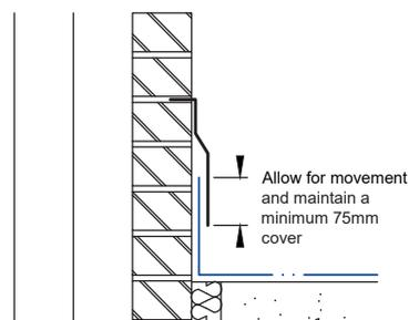
Where a timber frame structure abuts a masonry structure allowance should be made to accommodate movement in the timber frame and ensure the appropriate cover is maintained
