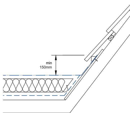
Upstand to decking and paving finishes e.g. where access is required
