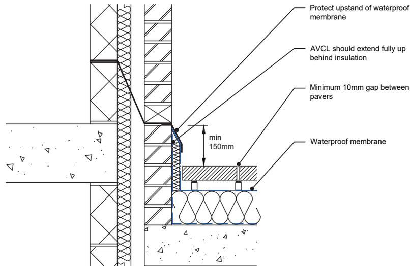
Timber frame construction where a lower level construction meets a brick outer leaf wall to roof abutment timber frame
