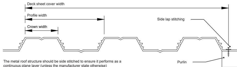
The metal roof structure should be side stitched to ensure it performs as a continuous plane layer (unless the manufacturer state otherwise)
